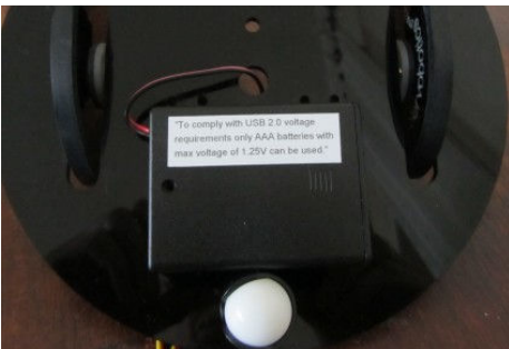
Glue the Velcron to the base plate by the ball caster.
