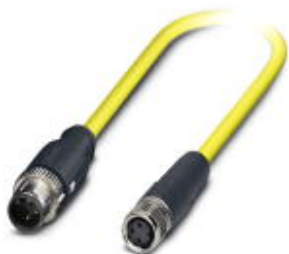
Sensor/Actuator cable, 3-position, PVC, yellow, shielded, Plug straight M12 SPEEDCON, A-coded, on Socket straight M8, Cable length: 0.5 m
