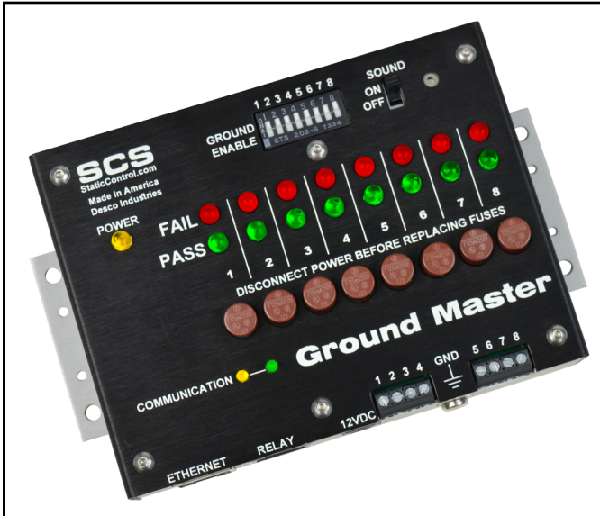
Figure 1. SCS 770060 Ground Master Monitor
