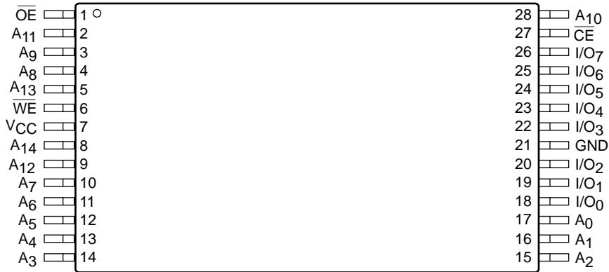
TSOP Top View (8mm X 13.4mm) (H)
