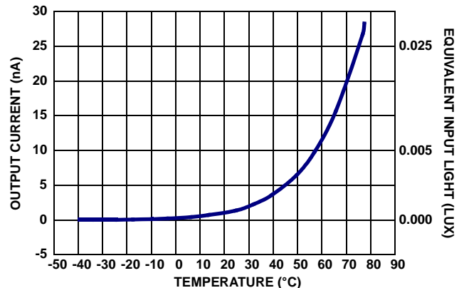
FIGURE 11. OUTPUT CURRENT vs TEMPERATURE AT 0 LUX
