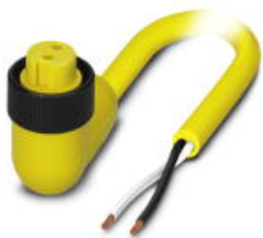
Power cable, 2-position, PVC, yellow, free cable end, on Socket angled 7/8"-16UNF, cable length: 2 m
