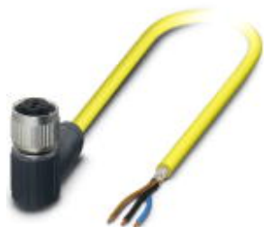
Sensor/Actuator cable, 3-position, PVC, yellow, shielded, free cable end, on Socket angled M12 SPEEDCON, A-coded, Cable length: 2 m
