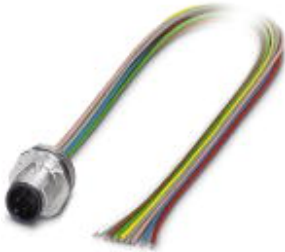
Sensor/Actuator flush-type plug, 8-pos., M12-SPEEDCON, A-coded, front/screw mounting with M16 thread, with 0.5 m TPE litz wire, 8 x 0.25 mm 2
