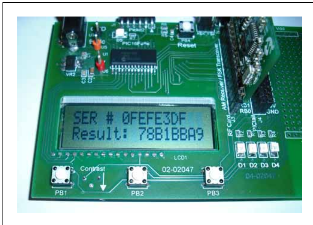
FIGURE 2-3: LCD SCREEN WITH DECODED INFORMATION
