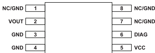
Package LE, 8-Pin eTSSOP Pinouts
