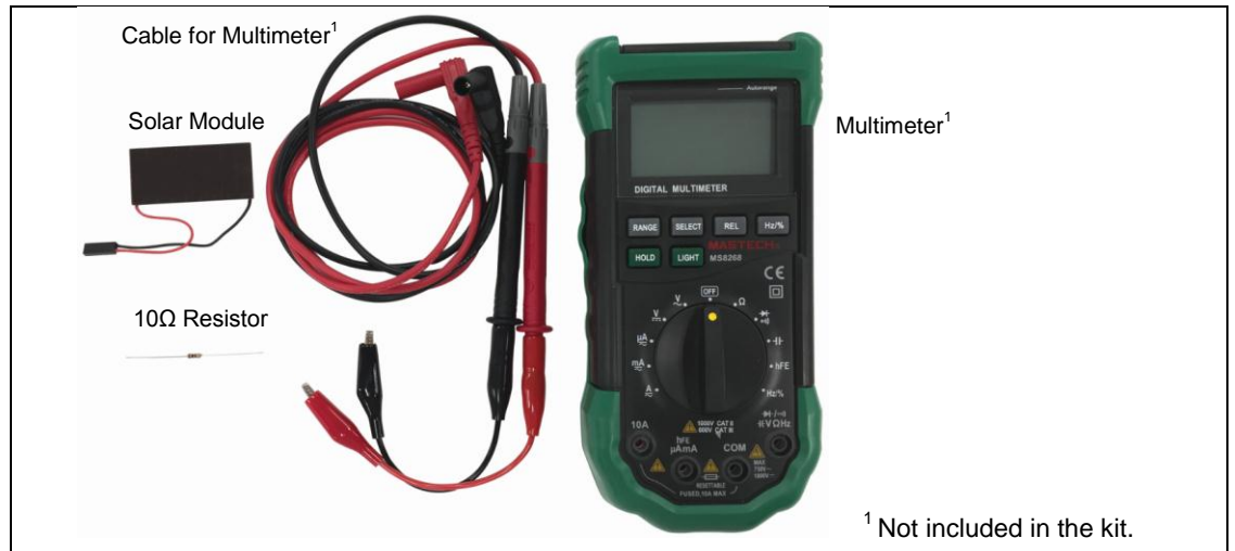
Figure 5-25. Components Required for Current Measurement
