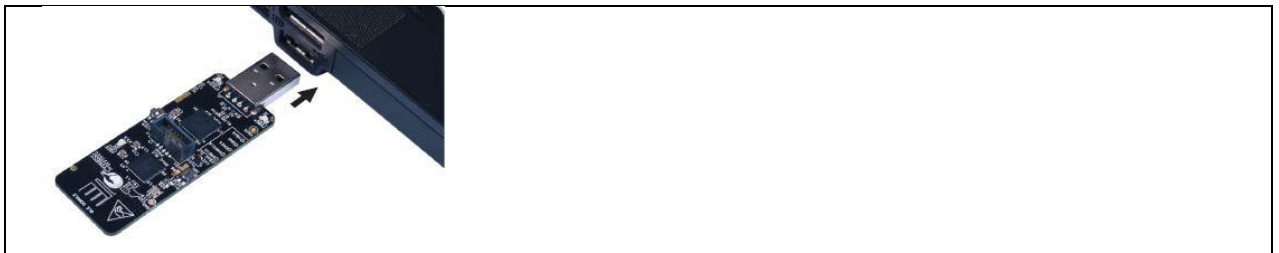
Figure 5-21. Connecting the USB Dongle to a PC USB Port
