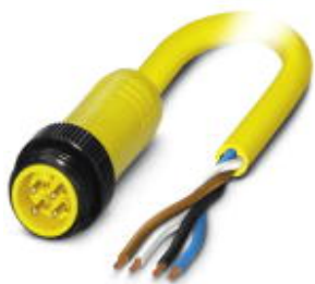
Power cable, 4-position, PVC, yellow, Plug straight 7/8"-16UNF, on free cable end, cable length: 2 m
