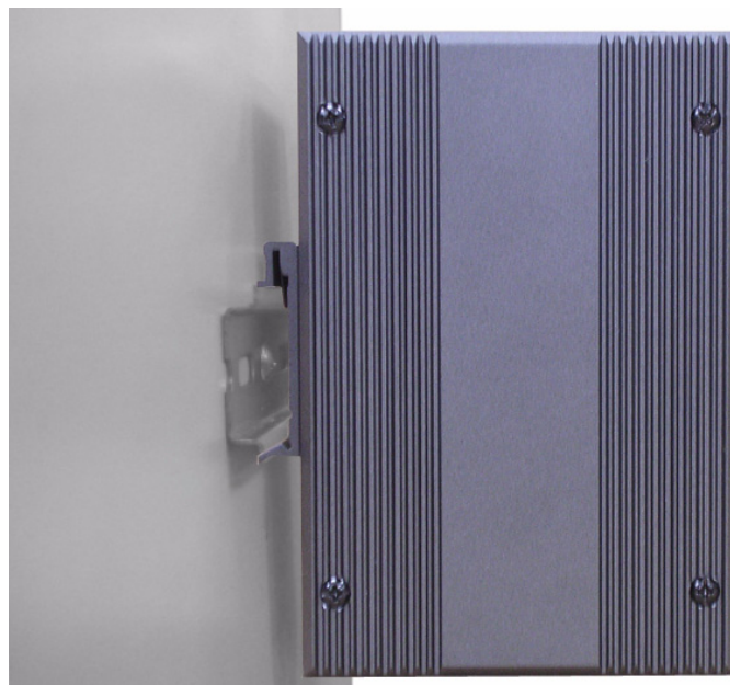
Figure 2.4 DIN-rail Installation Step 2
