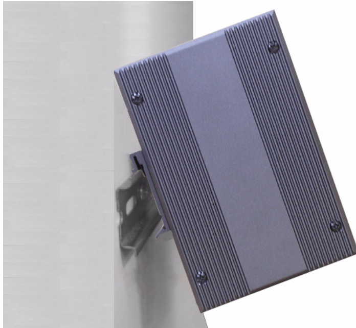
Figure 2.3 DIN-rail Installation Step 1
