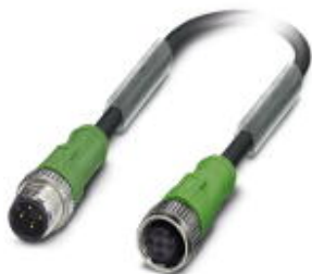
Sensor/actuator cable, 4-position, Variable cable type, Plug straight M12, A-coded, on Socket straight M12, A-coded, cable length: Free input (0.2 ... 40.0 m)
