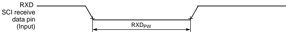
Figure 10-15 RXD Pulse Width
