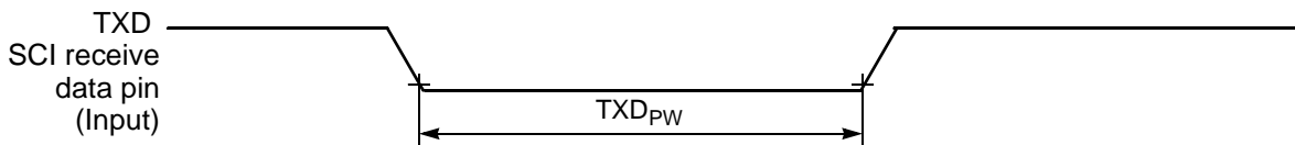
Figure 10-16 TXD Pulse Width
