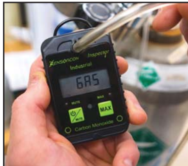
Connect the 50ppm calibration gas.
