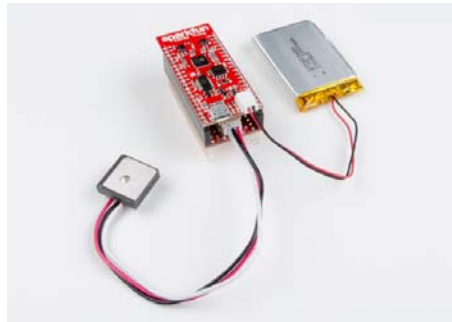
ESP32 Thing, motion shield, GPS receiver, and battery installed. The ESP32 Thing is ready for code!
