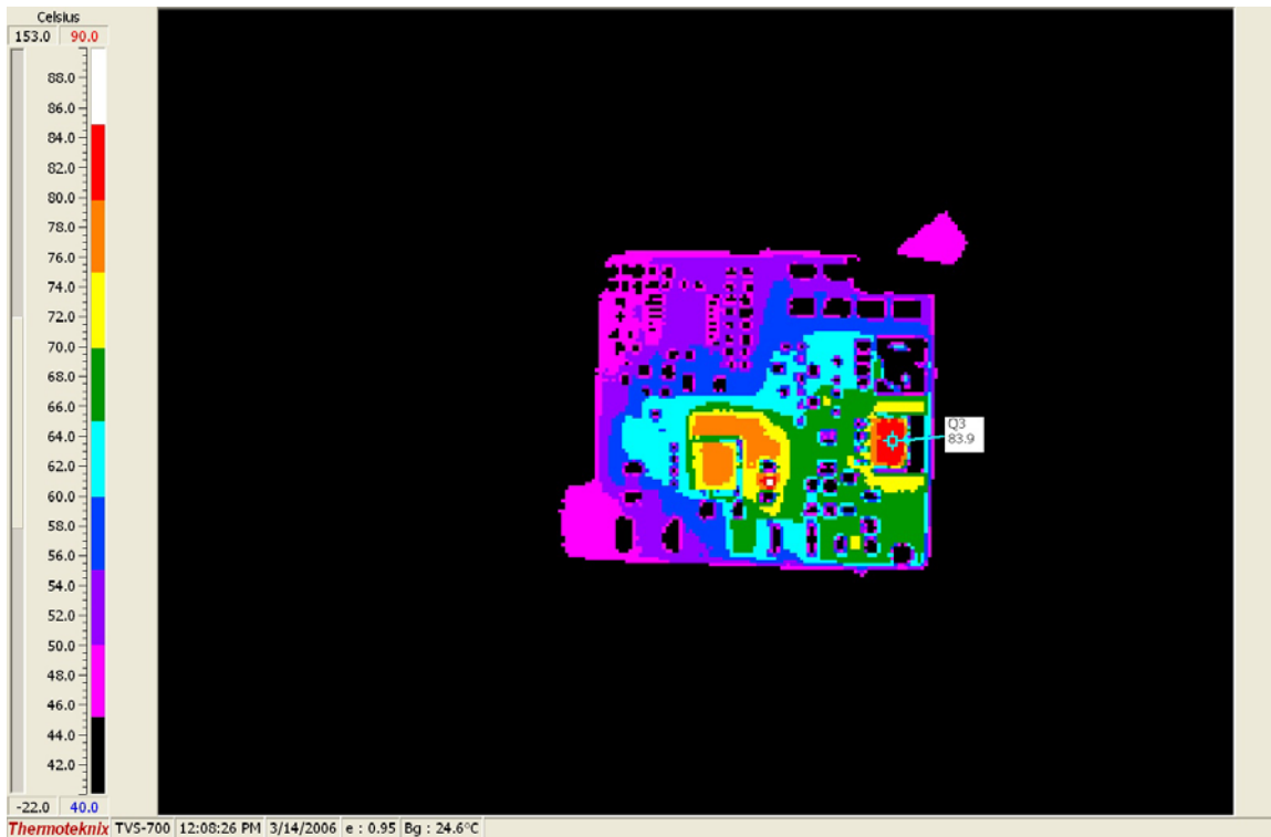
Figure 8. Temp Data (48Vin, 8A, 100LFM airflow – back)
