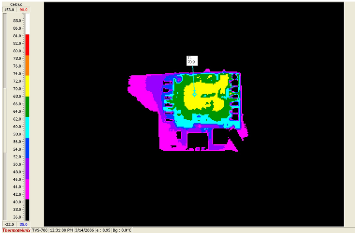
Figure 7. Temp Data (48Vin, 5A, 100LFM airflow – front)
