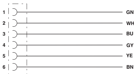
Contact assignment of 7/8" socket
