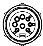
AISG 8-pin female interface with 4 loaded contacts
