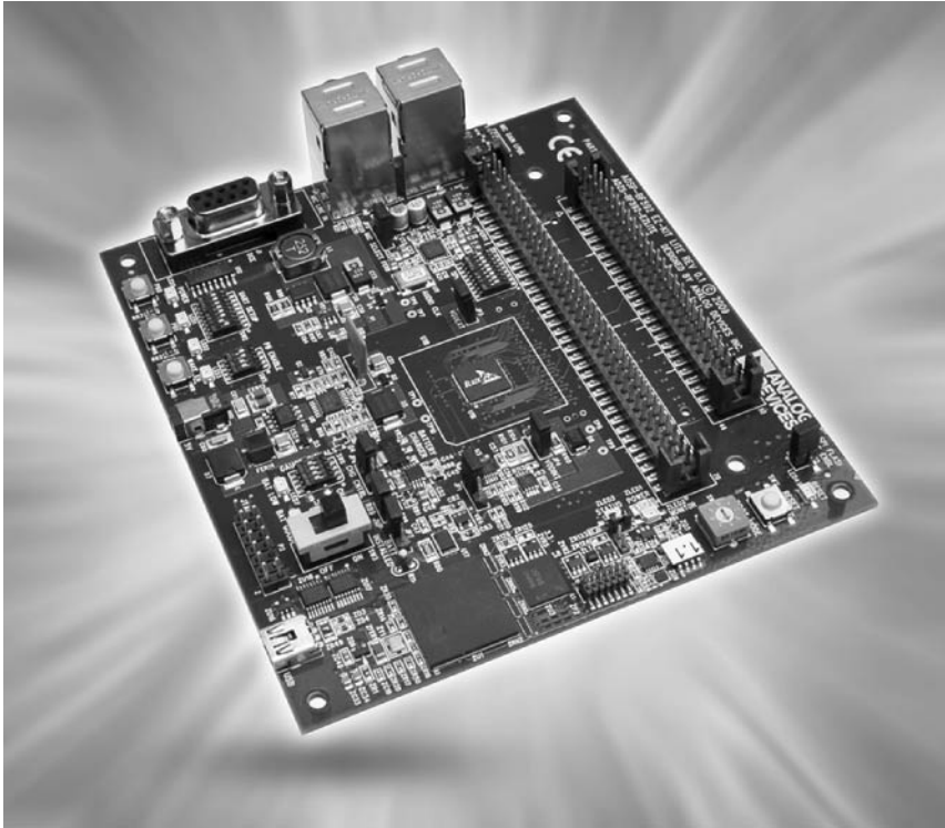
Figure 2-2. ADSP-BF592 EZ-KIT Lite Evaluation System
