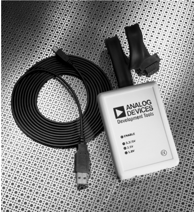
Figure 2-22. High-Performance USB 2.0 JTAG Emulator
