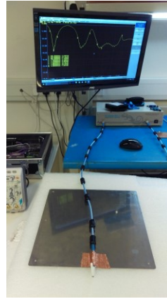
300mm x 300mm Ground Plane Edge
