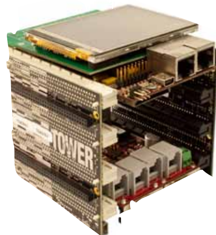
Figure 1. The TWR-MPC8309-KIT made up of the TWR-MPC8309, TWR-INDCTRL and TWR-ELEV modules. Mounted on the TWR-MPC8309-KIT is the optional MPC830x-TLCD module.
