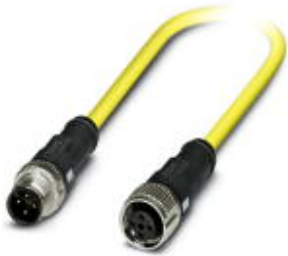
Sensor/Actuator cable, 4-position, TPE, yellow RAL 1021, Plug straight M12 SPEEDCON, A-coded, on Socket straight M12 SPEEDCON, A-coded, Cable length: 1.5 m
