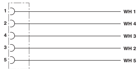
Contact assignment of the M12 socket
